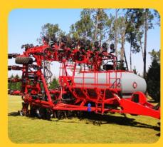
Multi sectional fold for optimal floatation and narrower transport widths
